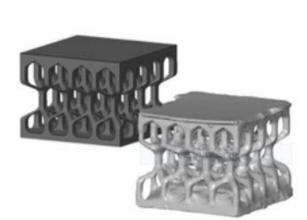
Combining reduction of a metal in the presence of light with 3D-printing enables 3D hybrid structures consisting of metal nanoparticles and organic polymers to be formed. This process is low in cost and rapid. The 3D structures produced have a multi-layered design. They can be used for energy dissipation purposes, such as in electronic device packaging.
