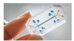
Current technologies like UV lithography, nanoimprint lithography and electron beam lithography can produce nanoscale features with low cost. The authors analysed the production of lab-on-a-chip devices through injection molding. Injection molding process parameters, feature dimensions and orientation relative to polymer flow direction were also examined. Finally the authors discuss the final product's compliance with technical specifications.
